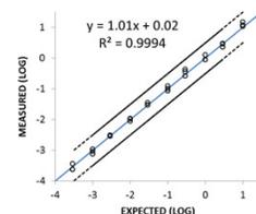
**Purpose:** Determine if three laboratories could measure cDNA reference samples within a half a log of expected answer.
